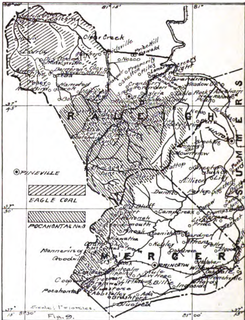
Figure 9.—Showing Probable Minable Area of Eagle and No. 3 Pocahontas Coals in Raleigh, Mercer and Summers Area.
